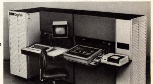
The GR 2270 in-circuit test system, designed for large printed circuit boards. It has the most flexible emulation and diagnostic software on the market. We also offer a powerful benchtop tester, the GR 2230 I, for smaller boards.
