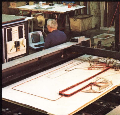
Computer-controlled wire harness and cable forming system cuts production time, test and rework costs up to 90%.
